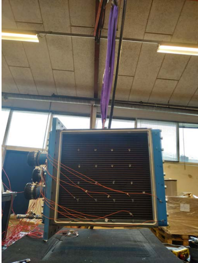
Heat exchanger under test simulating fixed boundary conditions
